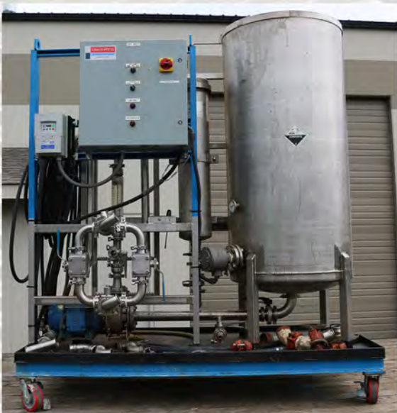
Chemical flushing system
