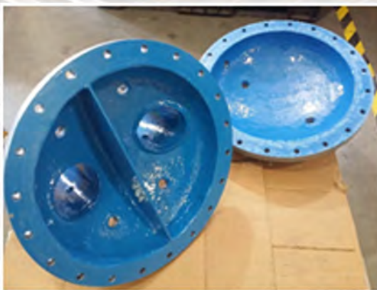
End cover coated repair
